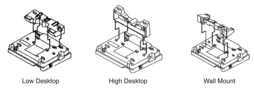
Figure 2-1 Footstand Mounting
