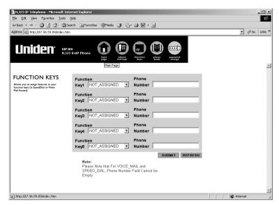
Figure 4-9 Function Key Configuration
