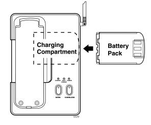
3. Make sure the BATTERY CHARGE LED lights. If it does not light, check to see that the AC adapter is plugged in, and that the battery pack is seated into the charging compartment.
